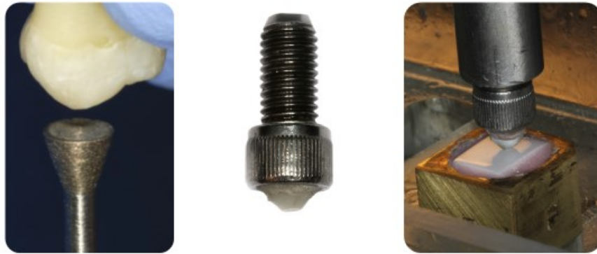
Figure 24 Antagonist preparation for “enamel wear” experiment. Bicuspids are altered with a diamond bur (left) and polished. Then mounted into a holder (middle). The enamel antagonist is then used in a pin-on-block design (right) with a sliding phase after initial contact.
